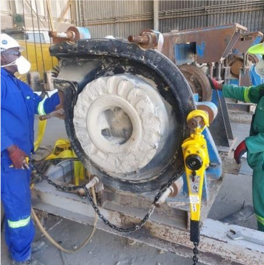
Successful stripping of slurry pump for refurbishment
