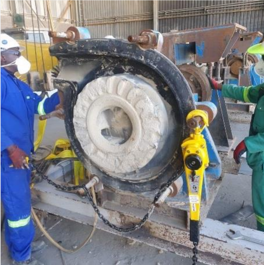
Successful stripping of slurry pump for refurbishment
