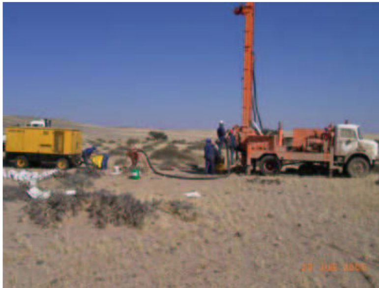
Figure 12: Drill rig on site. Super Rock 1000 rig adapted for RC drilling, towing a separate compressor
